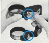
B. Loosen both clamp ring screws of the AF-400T 6x7 Bracket and detach the clamp rings from the bracket.
