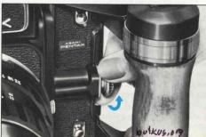
Adjustment of the Grip Angle: For flash photography the head grip can be angled in the direction of flash. Loosen the clamp ring screws at the top and bottom of the Grip with the accessory driver and turn the Grip so that the flash unit (accessory shoe) faces the direction desired, and retighten the screw. The clamp ring screws also feature a built-in lug for neck-strap attachment.
