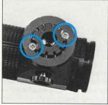
A. Remove the bracket clamp of the AF400T flash unit by loosening the two clamp screws and sliding the clamp off the neck.
